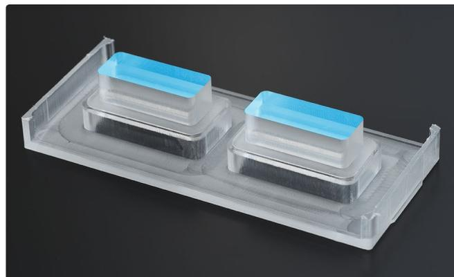
HoloLid placed in a Sarstedt 6-well plate (left). The areas marked blue are the observation windows which are immersed into the cell media (right).
