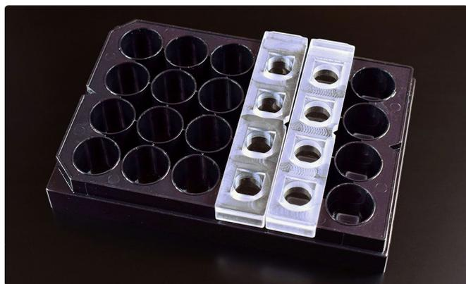
HoloLid placed on a ibidi  $\mu$ -Plate 24 well (left). The areas marked blue are the observation windows which are immersed into the cell media (right).
