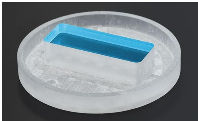
HoloLid placed on a Sarstedt 35 mm petri dish with the observation window immersed into the cell media (left). The area marked blue is the observation window which is immersed into the cell media (right).
