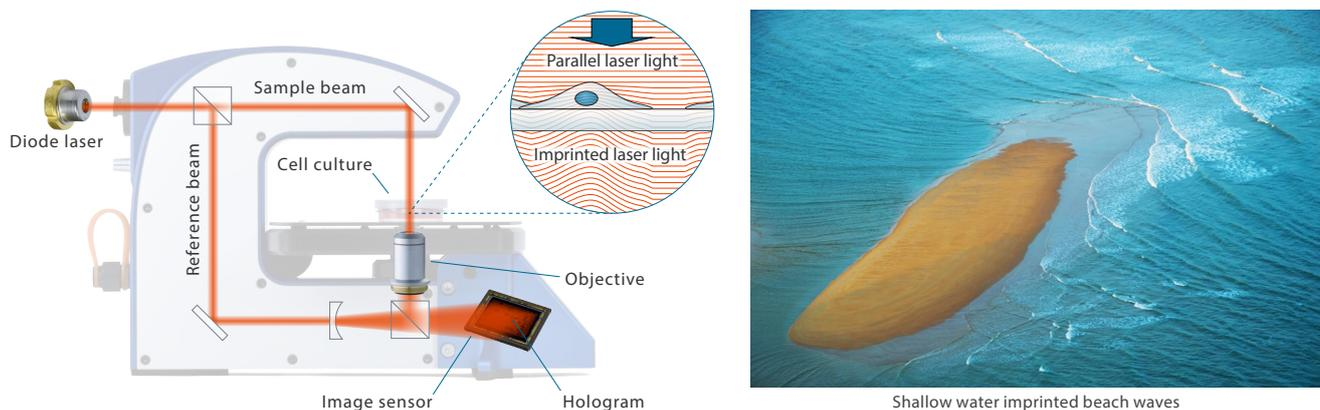
Holographic microscopy creates quantitative phase images by letting a sample beam and a reference beam interfere to create an interference pattern or *hologram*, as shown above. The hologram is recorded by an image sensor and computer processed to produce the phase image.
